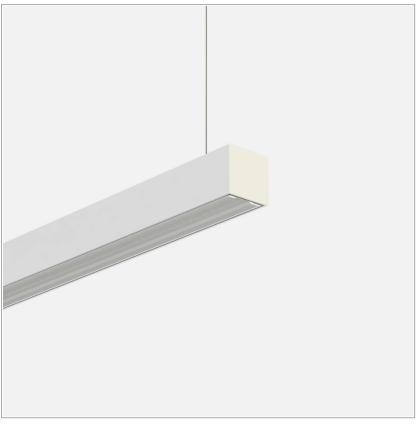
Linear lighting fixtures, in extruded aluminum 55x55mm, for ceiling, suspension. Embossed painted finish. Screens for diffused light in opal polycarbonate, for the PRO version are available optics with different beam openings. Might be equipped, if necessary, with spectra for horticulture. IP40 / IP43. Available default modules and modular system.
