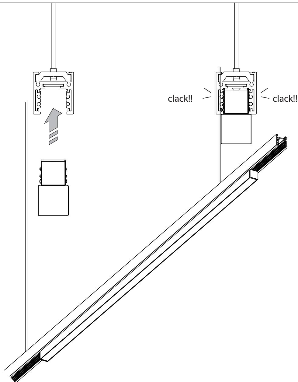
If the Microfile Track doesn't work, unhook the lamp from the track, turn it 180° and put it in the track again.
